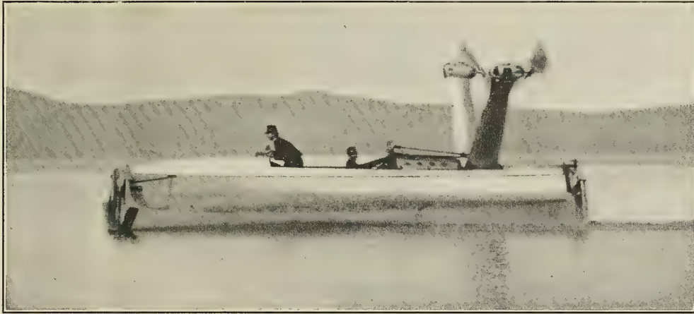
THE CROCCO-RICALDONI HYDROPLANE AT FULL SPEED ON TRIAL TRIP: HULL 18 INCHES OUT OF WATER.
